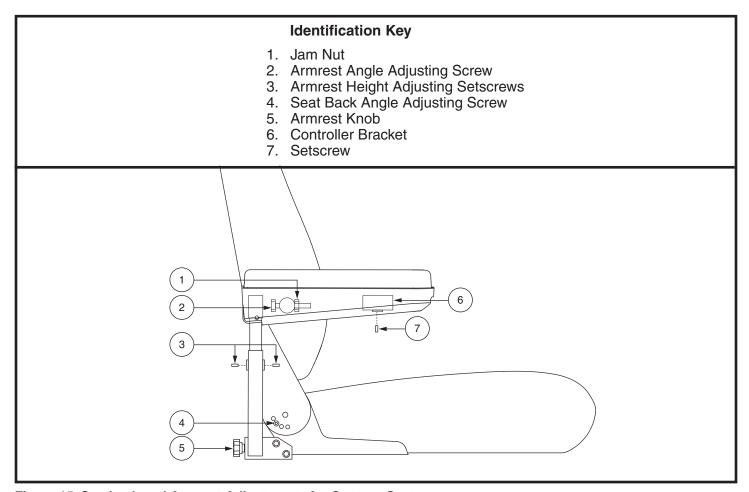
Figure 15. Seatback and Armrest Adjustments for Contour Seat
