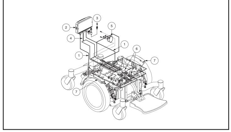
Figure 1. Q6 Series Electrical Components
