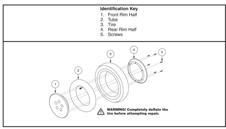
Figure 20. Q6 Series Drive Wheel Disassembled
