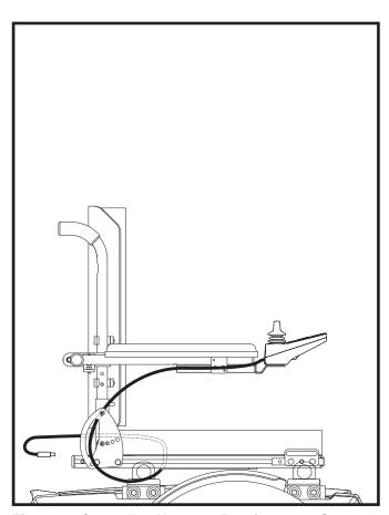
Figure 8. Controller Harness Routing on a Synergy Seat
