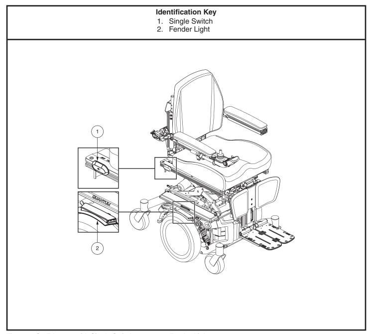
Figure 5. Q6 Edge 2.0 with Single Switch to operate Fender Lights.
