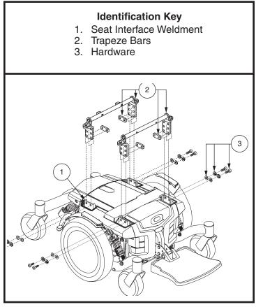
Figure 13. Seat Height/Angle Adjustment
