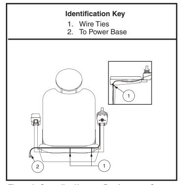
Figure 9. Controller Harness Routing on a Contour Seat
