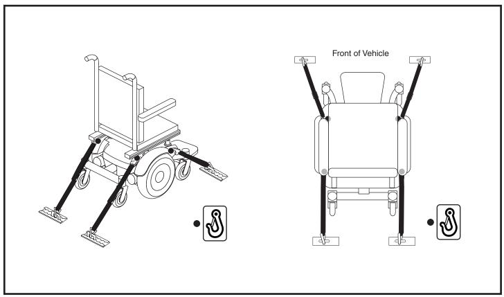
Figure 12. Unoccupied Transit System Securement Points
