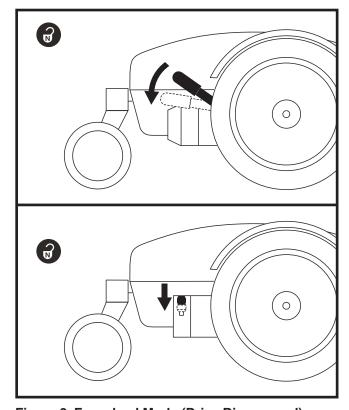
Figure 2. Freewheel Mode (Drive Disengaged)
