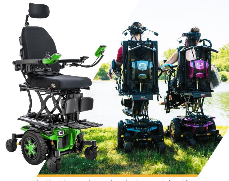
The Edge 3 has upgraded SRS (Smooth Ride Suspension) providing a smooth, comfortable ride and advanced stability. Optional iLevel is available at 7,2 km/h with up to 305 mm of power adjustable seat height. Standard features include LED fender lights, a USB charger, and drive wheel colour accents.
