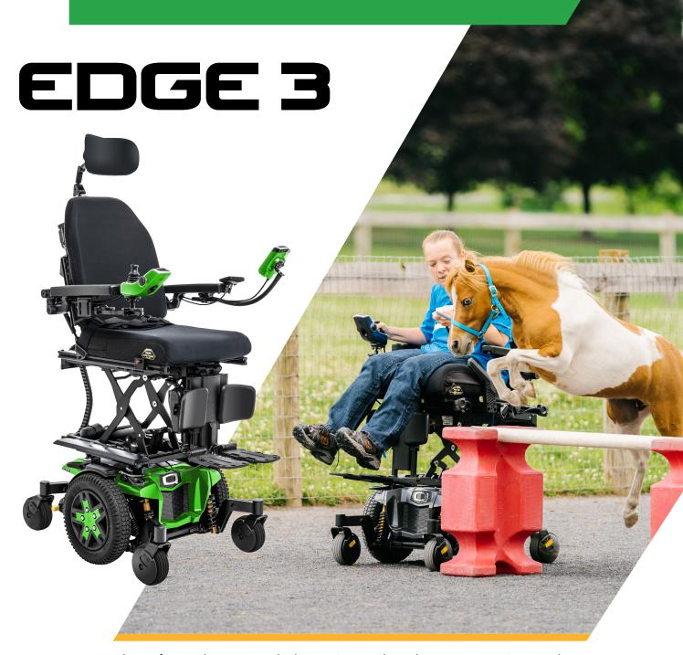
The **Edge 3** has upgraded SRS (Smooth Ride Suspension) providing a smooth, comfortable ride and advanced stability. Optional iLevel is available at 7,2 km/h with up to 305 mm of power adjustable seat height. Standard features include LED fender lights, a USB charger, and drive wheel colour accents.
