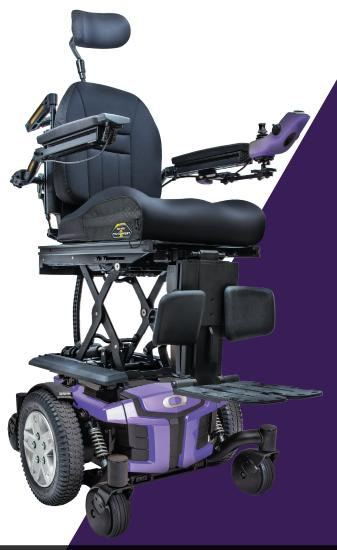
With features like standard 4-pole motors, Mid-Wheel 6 Drive Design and ATX Suspension, the **Q6 Edge HD** is engineered to meet the performance needs of the most active user. The Q6 Edge HD accepts a complete range of seating and electronics options to deliver exceptional rehab capability at an excellent value, and is available with our iLevel technology.
