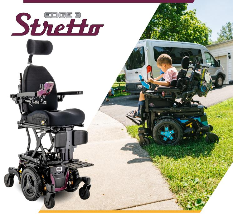
The Q6 Edge 3 Stretto features a narrow width for outstanding maneuverability and is equipped with independent SRS (Smooth Ride Suspension), making it ideal for children, teenagers and small adults. The Stretto is available with 12,5" or 14" drive wheels and optional 305 mm of iLevel power-adjustable seat height.
